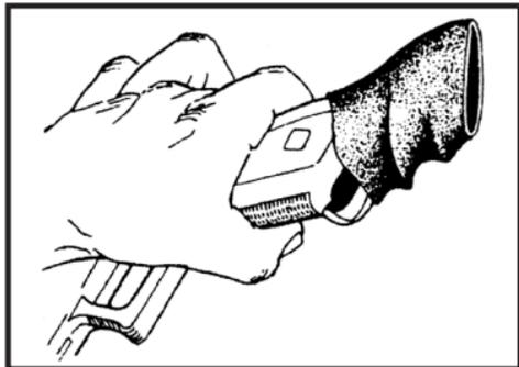
**2.** Begin by holding the firearm as shown. At the rearmost corner, cover the frame with the HANDALL Jr. Make sure it is right side up. Look for the (up) inside the grip.
