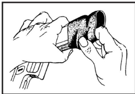
**3.** Next, pull the sleeve towards the front of the firearm until the finger groove ridge is over the front corner of the frame. The HANDALL Jr. is designed to fit tightly and much force may be required to complete this step. The sleeve should be stretched as evenly as possible. The rubber is very durable and tear resistant although care must be exercised not to gouge, cut, or pull excessively on the edges of the sleeve, as a tear may develop.
