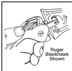
**6** Mate the firearm frame and **MONOGRIP** by first placing stirrup and pin(s) into the internal guide grooves.
