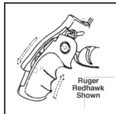
**7** The **MONOGRIP** should be guided up behind the trigger guard, then using a radial motion, fully seat the frame into your **MONOGRIP**. It must be fully seated on the frame before inserting mounting screw.
