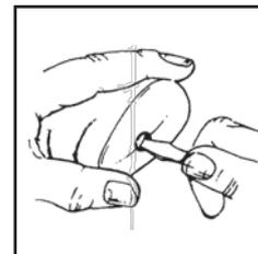
**8** Insert mounting screw through the hole on bottom of the grip. Insert screw so it enters stirrup threads, and using the appropriate screwdriver, tighten screw until snug, no tighter. Over-tightening does nothing to increase grip tightness and can damage the screw or stirrup.
