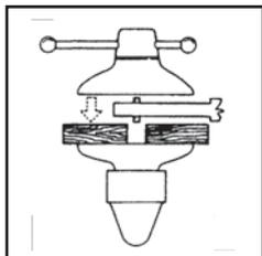
**4** Remove grip pin(s) or lug(s) by using hammer and punch, or bench vise and block of wood or other shim as shown.
