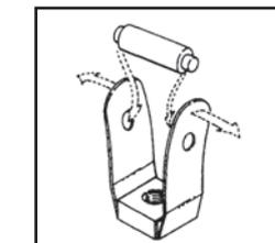
**2** The stirrup is made from spring steel and will spread from pin for removal and installation. Spread stirrup and take pin out.
