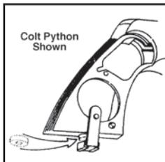
**5** Install stirrup as pictured. For Blackhawk models use lowest stirrup pin for your frame type. Take screw out of stirrup. If a spacer is included with your grip, insert it between the stirrup and bottom strap as shown.
