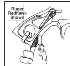
**9** Your **MONOGRIP** is designed to fit an average size firearm frame, however, frame dimensions do vary from firearm to firearm. If necessary your **MONOGRIP** can be adjusted by placing small shim(s) of tape on the lower corner of the front strap. Add or subtract tape until grip is flush with backstrap.
