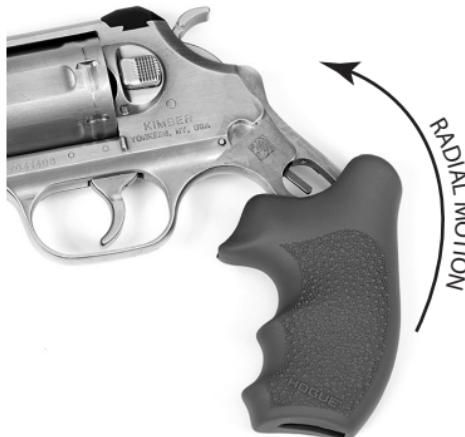
**5. It is unnecessary to remove your Hogue rubber K6s grip for routine cleaning. If you need to take it off for further maintenance, spread the bottom of the grip with the included Hogue Bantam tool. Fully insert it into the bottom of the frame and slide the grip off while the tool is engaged.**
